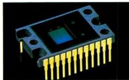
Figure 3. The charge-coupled device image sensor is a complicated device built in an integrated circuit configuration. (Courtesy of BTS.)
